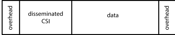
Fig. 1. Example fixed-length packet showing overhead, data, and CSI dissemination. The CSI dissemination consists of M channel estimates and each channel estimate (including its associated timestamp) has a length of one word. The data and overhead consists of D words. The total packet length is P = D + M words.
